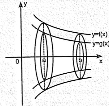
$$f(x) \geq g(x) \Rightarrow V_x = \pi \int_a^b (f^2(x) - g^2(x)) dx$$
